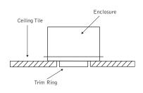
Figure 8. Enclosure and trim ring side view
